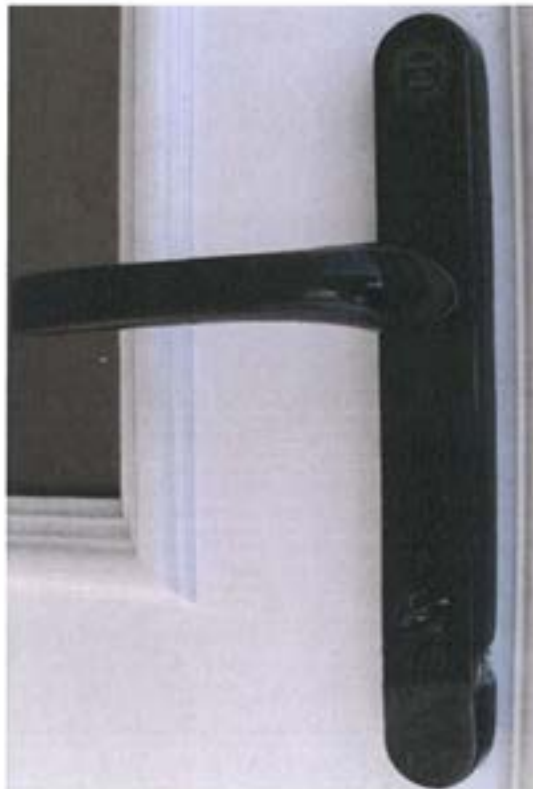
Sample following Annex A part 1 attack testing
